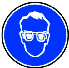
*Warning:* to avoid any risk of injury due to eventual projections when using an automated machine tool, including in manual mode, **you must imperatively wear safety eyeglasses.**
